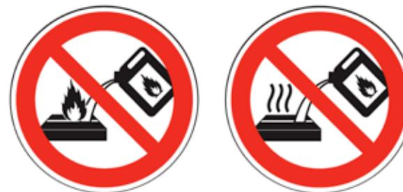
**2.10** Do not fill the burner when it is still in use or when it is still hot.
