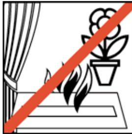
**2.15** Do not place the burner near easily flammable objects.
